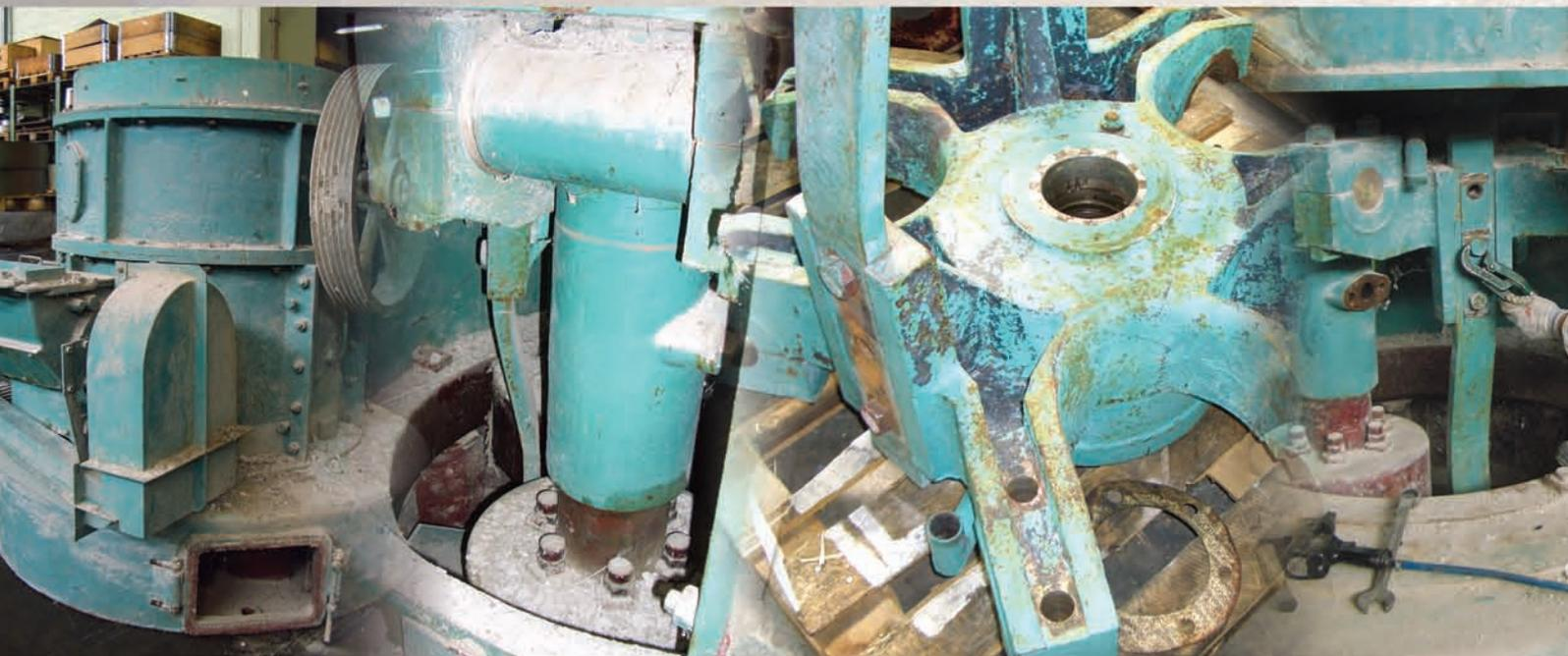
Successful grinding tests were carried out on Dec. 15, 2006 with 3 t of limestone. The NEA pendulum roller mill with a radial classifier could easily achieve 99% < 30 µm for a throughput of 2.1 t/h Rollovit and 95% < 120 µm with 5.7 t/h Filler. Exactly the requirements for later production under real conditions.
